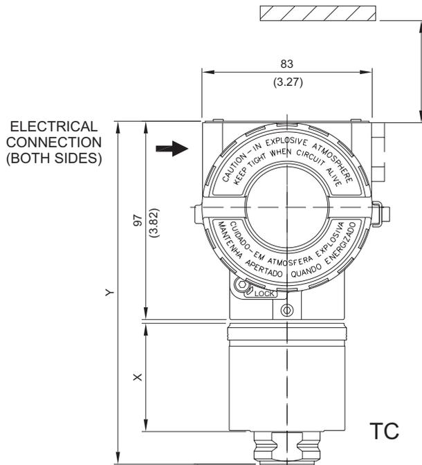
Allow 150 mm minimum for local zero and span adjustment with magnetic tools
